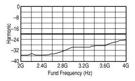
Figure 6. Harmonics vs. Frequency
