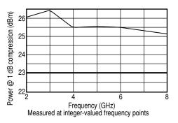
Figure 4. Power Output vs. Frequency
