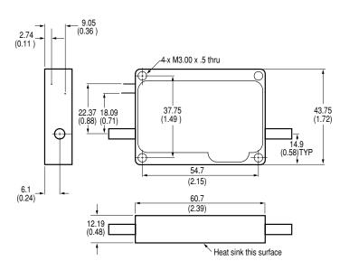
Figure 3. Agilent 87400A outline drawing. Dimensions in millimeters and (inches).
