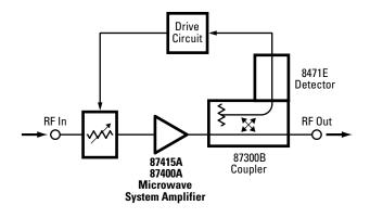
Figure 1. External leveling looping
