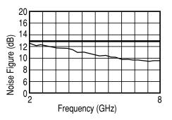
Figure 7. Noise Figure vs. Frequency
